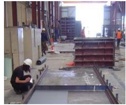
Left: Full height concrete channels, to be used as column formers. Above: Making up of panel moulds.
