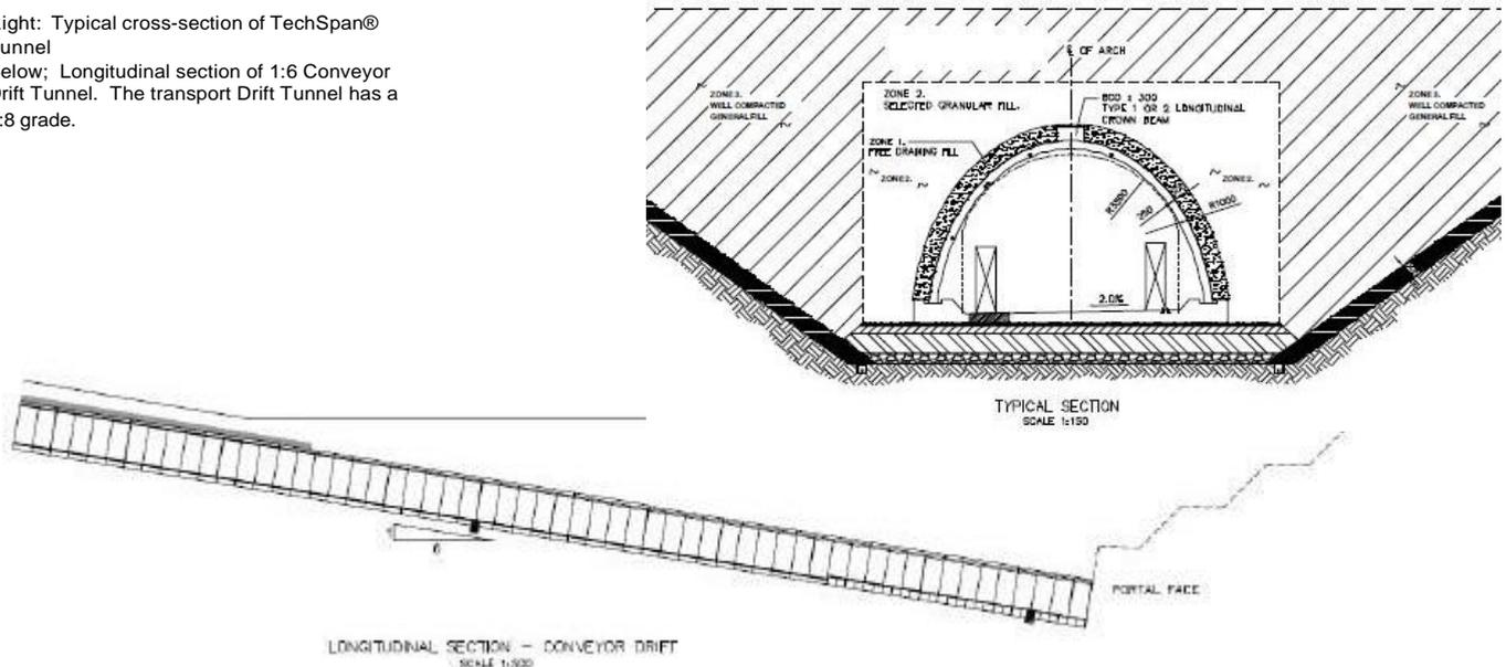
connectors to maintain longitudinal stability of the arch units. Due to transport capacity limitations placing each of the footing units at 25 tonnes, their width was limited to 1.1m and because the units are so narrow, these in-situ shear connectors needed to be included to prevent rotation.”
